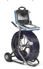
Designed for small to medium municipalities, this manhole-to-manhole inspection system is suitable for 4"–12" lines. Additional features include a 12" daylight readable screen, all-digital recording and wireless streaming to any mobile device. The PGR400's 1-1/2" diameter self-leveling camera head produces crystal-clear color imagery and has a 512Hz sonde transmitter built in.
